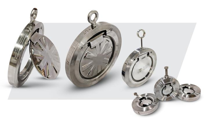
Our latest addition in Swing Plate Check valve is Specialized Enginnered Valve with Seat in PTFE / TFM and Valve Body/Disc in all Exotic Alloys like HAESTALLOY C-22, R-55, S.S904-L, ALLOY-20, DUPLEX S.S.316/S.S.316-L. This Valve MOC is selected in consultation with the Buyer makes it an ideal Check valve for all their Corrosive and Solvent application Services where standard Elastomer / Rubber Seat, Metal to Metal Seat is not suitable.
