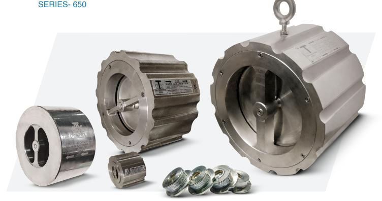
TDK offers Wafer Type Axial Check Valves specifically designed for fast-reversing systems where backflow is a constant concern .Spring loaded Double Guided Disc ensure immediate stoppage of flow before pump stops completely .This prevents flow reversal & water hammer, and ensure Valve close rapidly without slamming.
